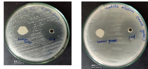
Fig: 6 Analysis of Antimicrobial efficacy (a. E. coli & b. Candida albicans ) on Viscose and cotton blend fabric
