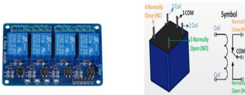
Figure 6: The relay and its characteristics
