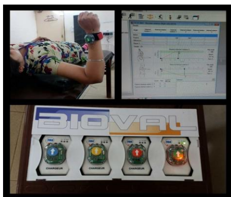
Figure 3: Starting Position Of Shoulder For Measuring Rotation Range Of Motion Using Motion Analyzer Sensors With Motion Analyzer Software: R M ingenierie Sy Co Mo Re version 8.52.0 And Bioval sensors.
